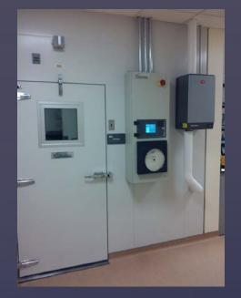
> Designed to control temperature and humidity
