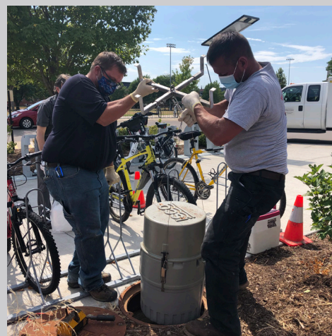
Plumbers retrieve a composite flow-weighted sampling unit from a campus wastewater manhole. UW-Madison is monitoring campus wastewater as part of a statewide SARS-CoV-2 wastewater surveillance network.
